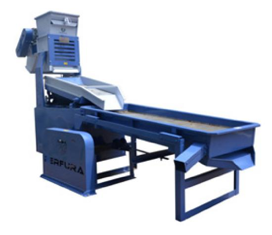
**5. Grain Polisher:** Grain Polisher is used for semi polishing millets like Little, Kodo, Foxtail, Proso, Barnyard, Finger, Pearl Millet & Sorghum. The degree of polished is based on the amount of time the grain is withheld inside the polishing chamber. Specifications: Capacity: 350 kg/hr; Power Requirement: 3HP Motor.
